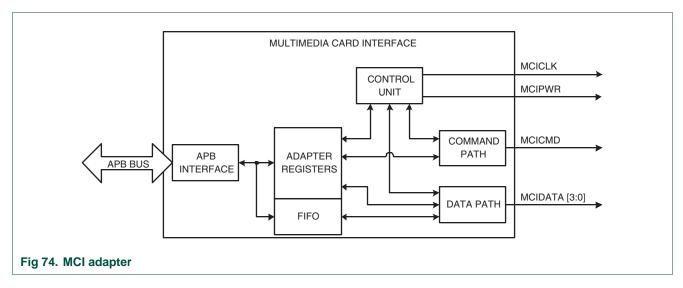
The MCI adapter is a multimedia/secure digital memory card bus master that provides an interface to a multimedia card stack or to a secure digital memory card. It consists of five subunits:
