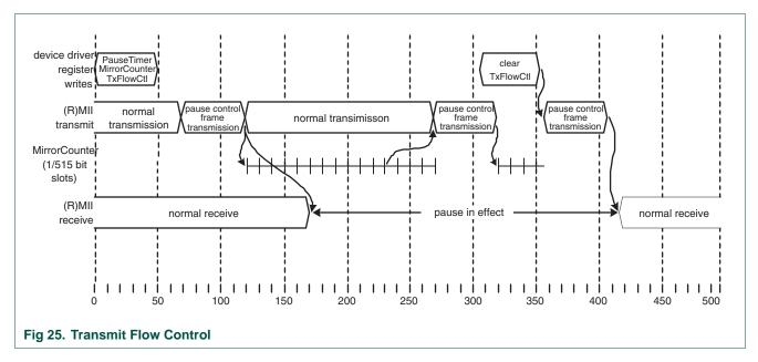
In this example, a frame is received while transmitting another frame (full duplex.) The device driver detects that some buffer might overrun and enables the transmit flow control by programming the PauseTimer and MirrorCounter fields of the FlowControlCounter register, after which it enables the transmit flow control by setting the TxFlowControl bit in the Command register.
