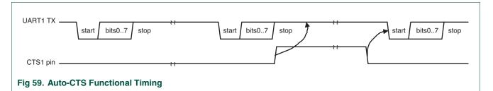
While starting transmission of the initial character the CTS1 signal is asserted. Transmission will stall as soon as the pending transmission has completed. The UART will continue transmitting a 1 bit as long as CTS1 is deasserted (high). As soon as CTS1 gets deasserted transmission resumes and a start bit is sent followed by the data bits of the next character.
