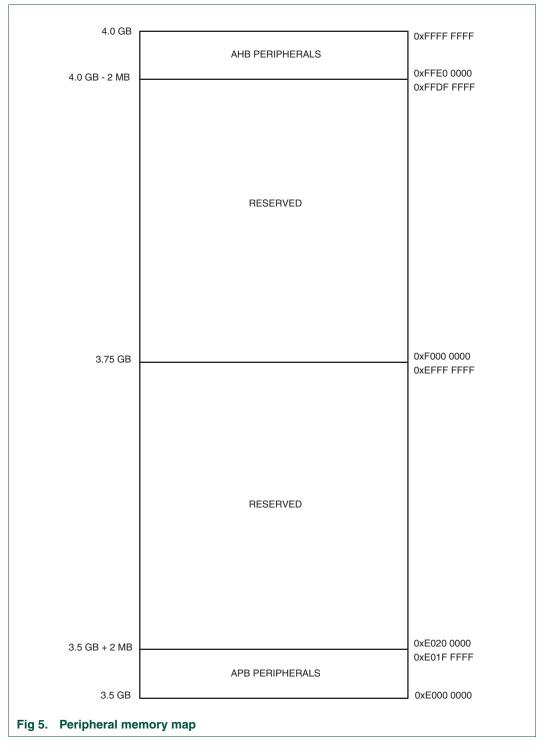
Figure <u>6</u> and <u>Table 2–4</u> show different views of the peripheral address space. Both the AHB and APB peripheral areas are 2 megabyte spaces which are divided up into 128 peripherals. Each peripheral space is 16 kilobytes in size. This allows simplifying the address decoding for each peripheral.
