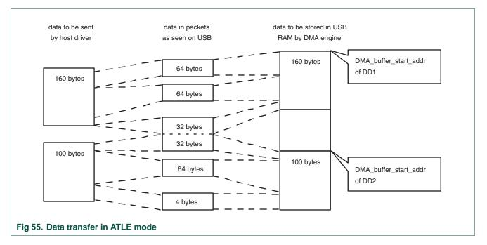
Figure 13–55 shows a typical OUT USB transfer in ATLE mode, where the host concatenates two USB transfers of 160 bytes and 100 bytes, respectively. Given a MaxPacketSize of 64, the device hardware interprets this USB transfer as four packets of 64 bytes and a short packet of 4 bytes. The third and fourth packets are concatenated. Note that in Normal mode, the USB transfer would be interpreted as packets of 64, 64, 32, and 64 and 36 bytes.
