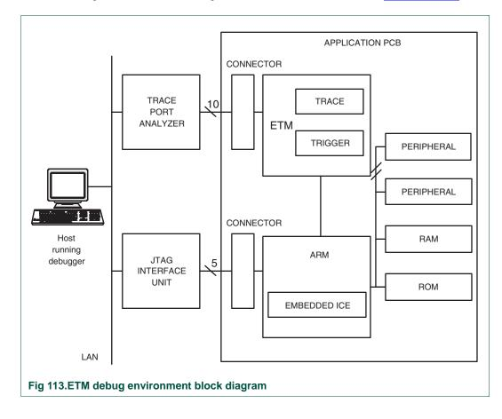
The block diagram of the ETM debug environment is shown below in Figure 30–113.
