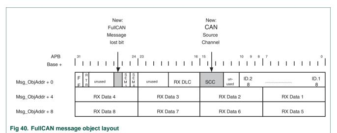
The new message lost bit (MsgLst) is introduced to indicate whether more than one FullCAN message has been received since last time this message object was read. For more information the CAN Source Channel (SCC) of the received FullCAN message is added to Message Object.
