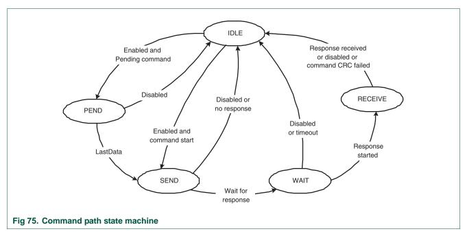
When the WAIT state is entered, the command timer starts running. If the timeout<sup>1</sup> is reached before the CPSM moves to the RECEIVE state, the timeout flag is set and the IDLE<sup>2</sup> state is entered.
