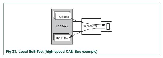
A message transmission is initiated by setting Self Reception Request bit (SRR) in conjunction with the selected Message Buffer(s) (STB3, STB2, STB1).
