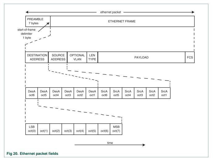
Figure 11–20 illustrates the different fields in an Ethernet packet.
