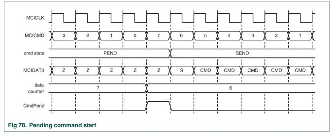
The data block counter determines the end of a data block. If the counter is zero, the end-of-data condition is TRUE (see <u>Section 18–5.10 "Data Control Register (MCIDataCtrl</u> - <u>0xE008 C02C)</u>" for more information).
