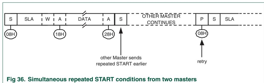
Fig 36. Simultaneous repeated START conditions from two masters
