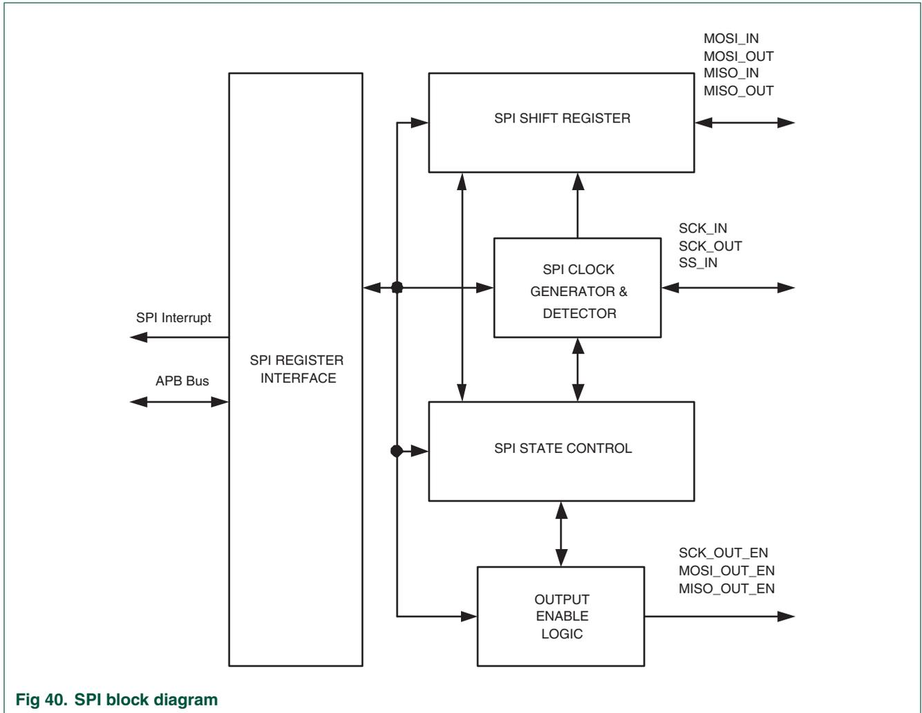
Fig 40. SPI block diagram
