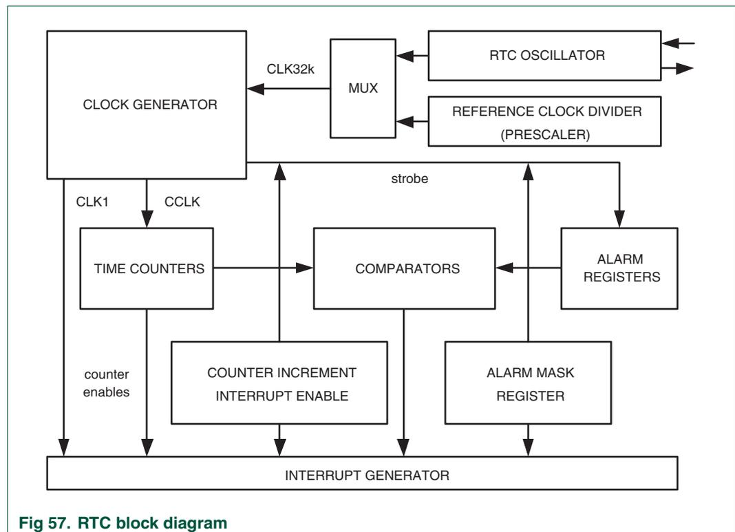
Fig 57. RTC block diagram
