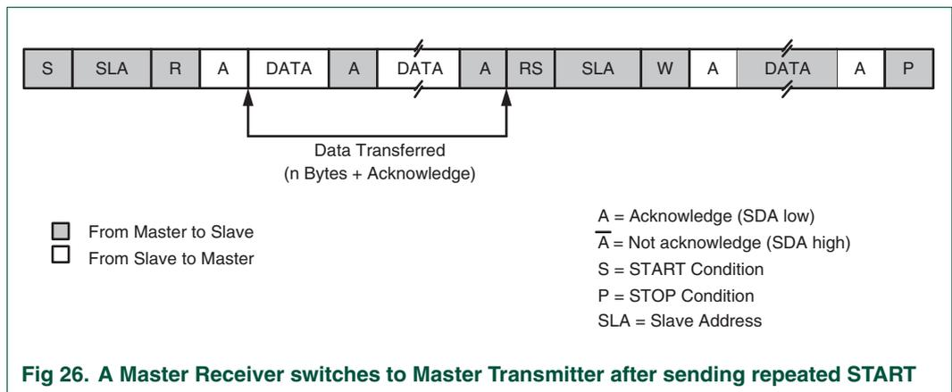
Fig 26. A Master Receiver switches to Master Transmitter after sending repeated START
