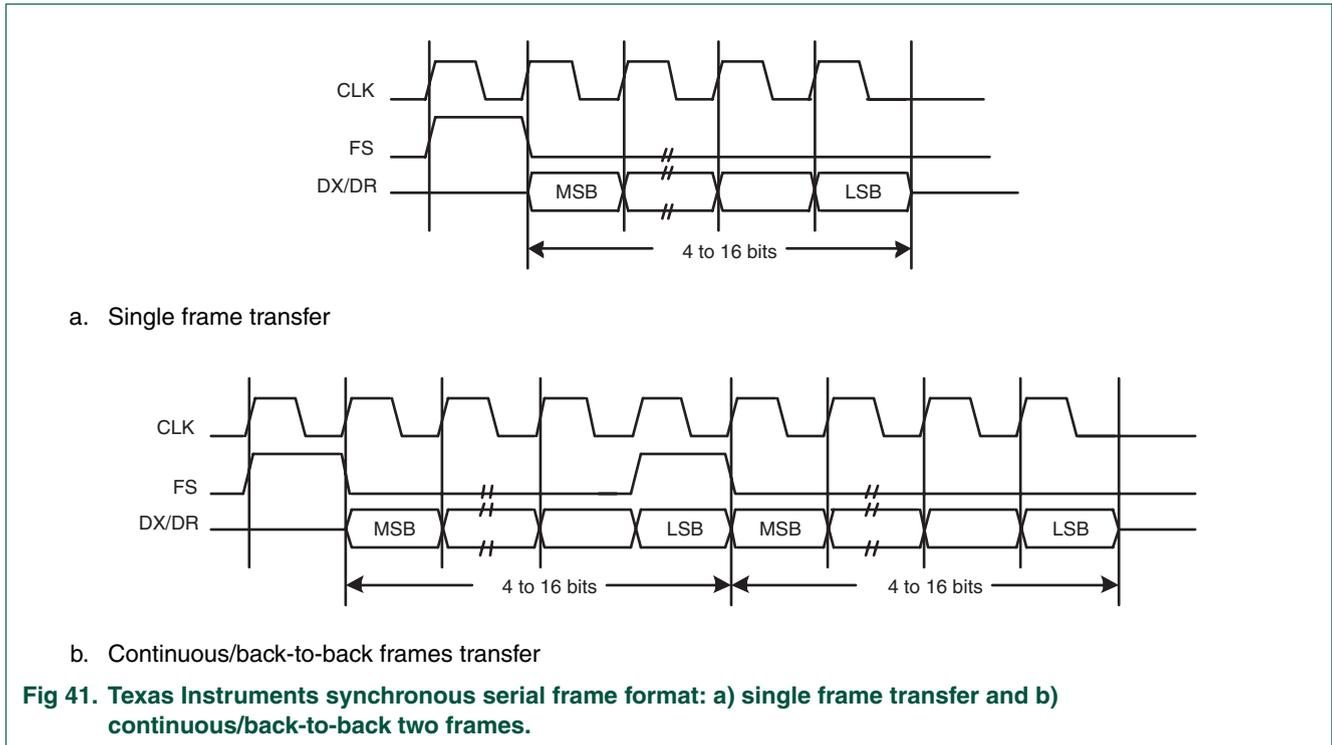
**Fig 41. Texas Instruments synchronous serial frame format: a) single frame transfer and b) continuous/back-to-back two frames.**
