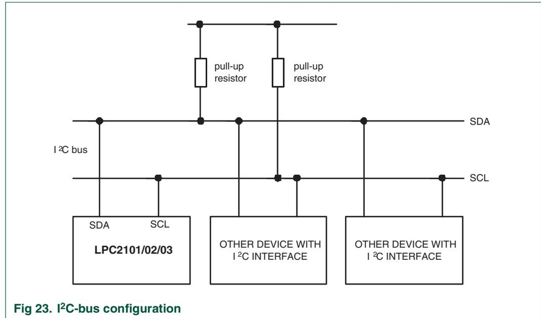
Fig 23. I<sup>2</sup>C-bus configuration
