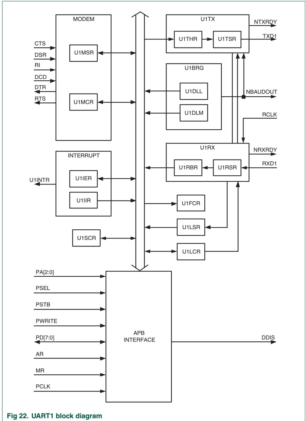
Fig 22. UART1 block diagram
