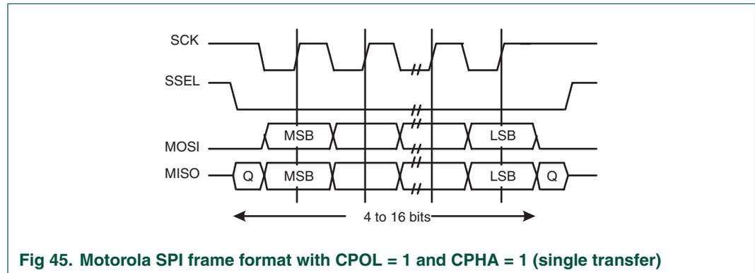
Fig 45. Motorola SPI frame format with CPOL = 1 and CPHA = 1 (single transfer)
