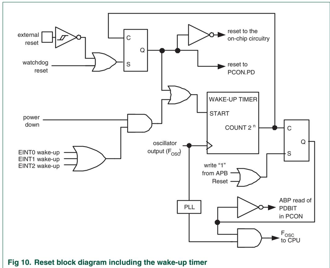
Fig 10. Reset block diagram including the wake-up timer
