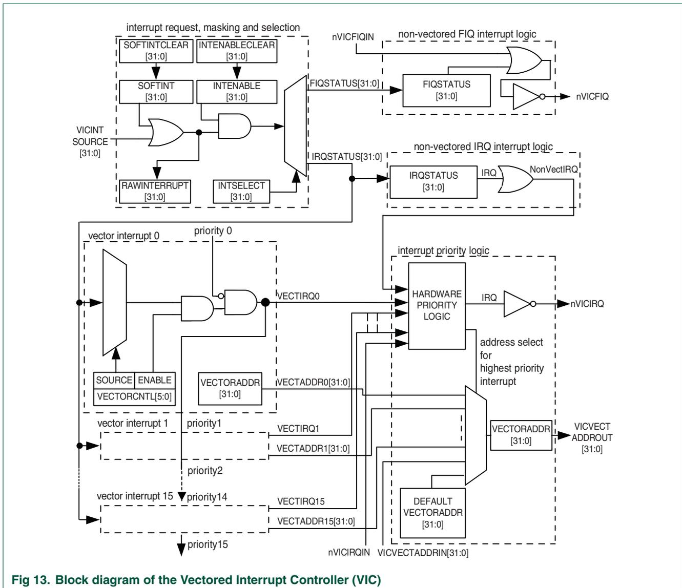
Fig 13. Block diagram of the Vectored Interrupt Controller (VIC)
