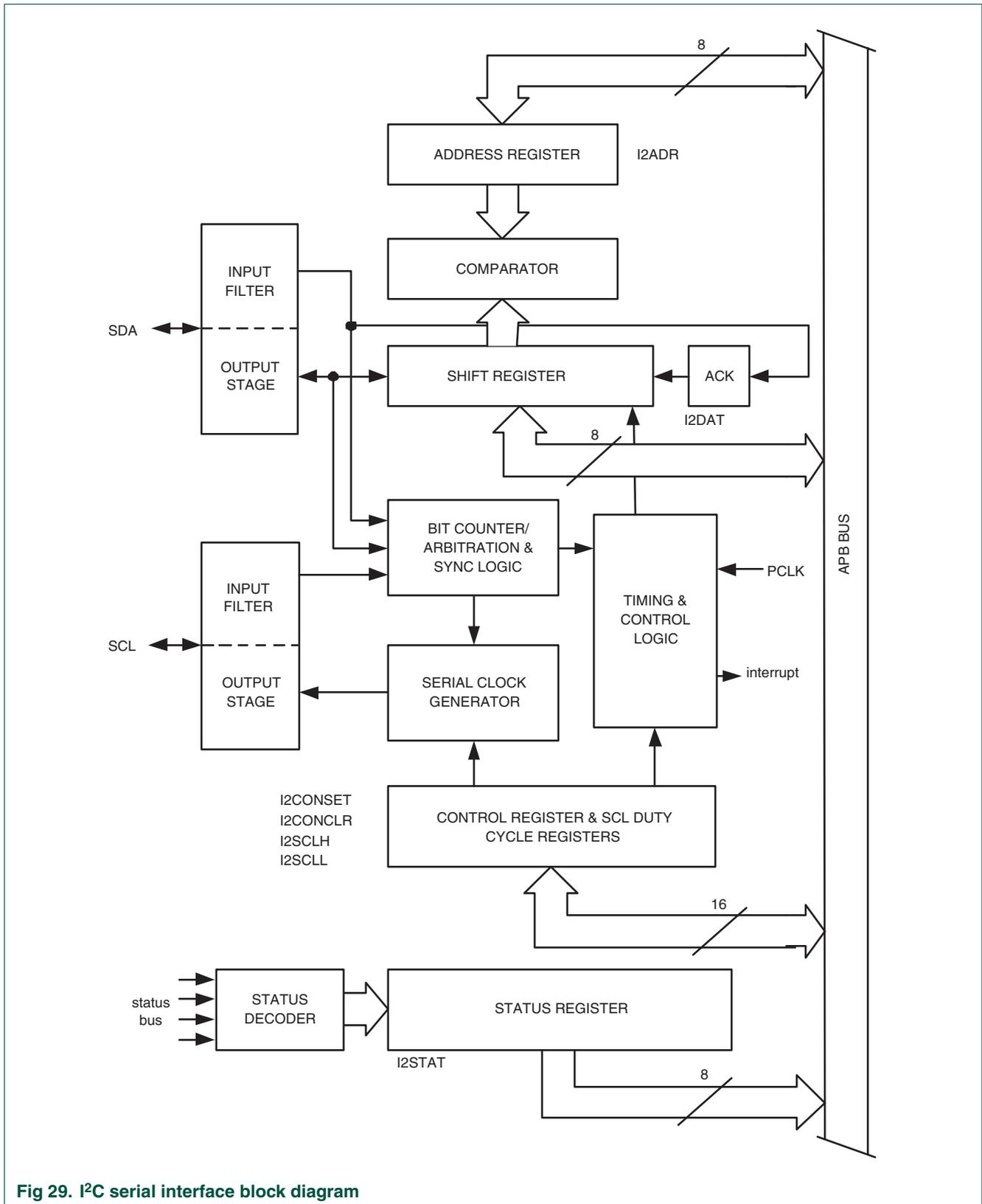
Fig 29. I<sup>2</sup>C serial interface block diagram
