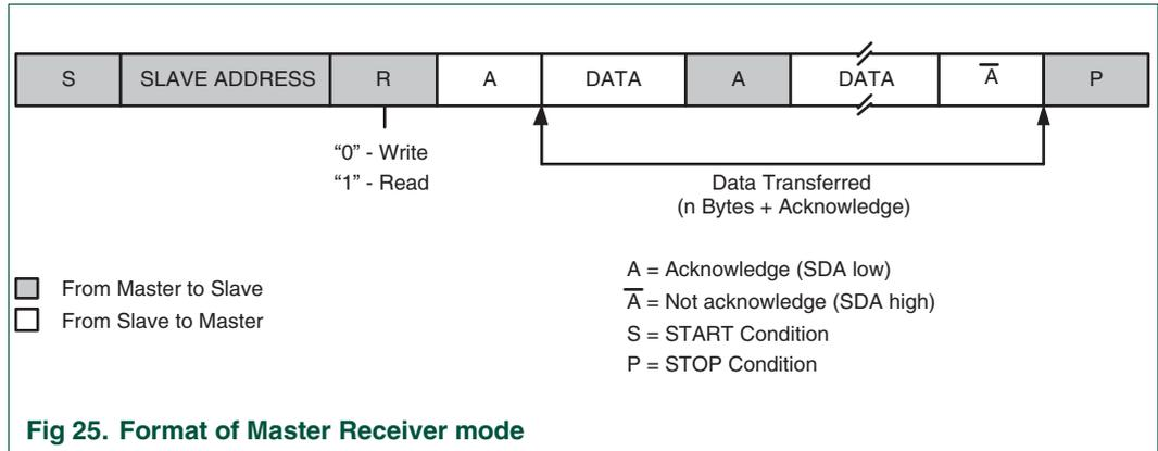
Fig 25. Format of Master Receiver mode
