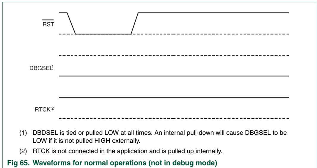
Fig 65. Waveforms for normal operations (not in debug mode)
