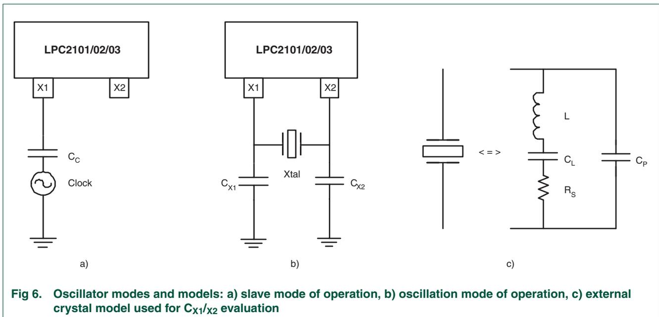
Fig 6. Oscillator modes and models: a) slave mode of operation, b) oscillation mode of operation, c) external crystal model used for  $C_{X1/X2}$  evaluation
