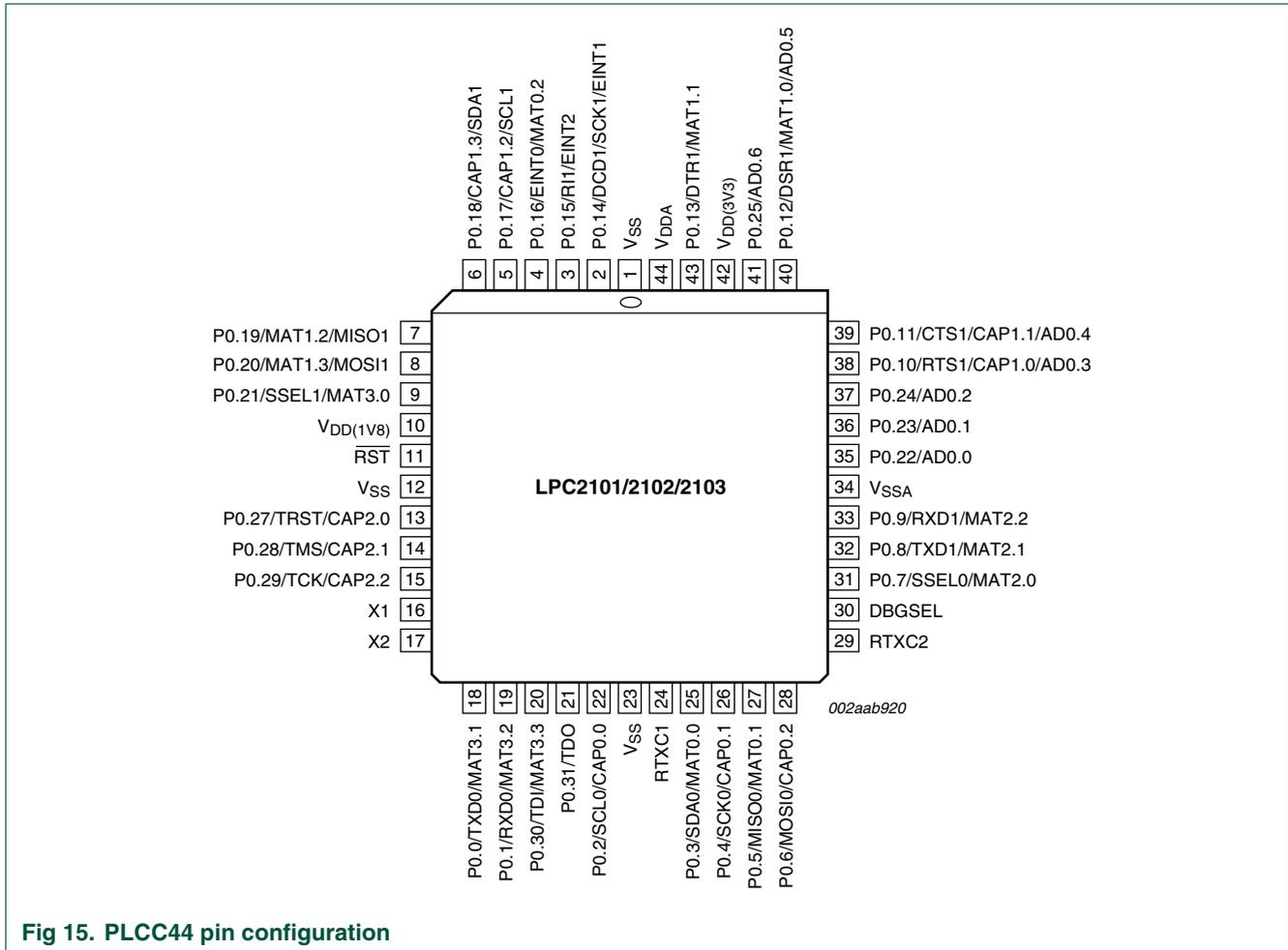
Fig 15. PLCC44 pin configuration
