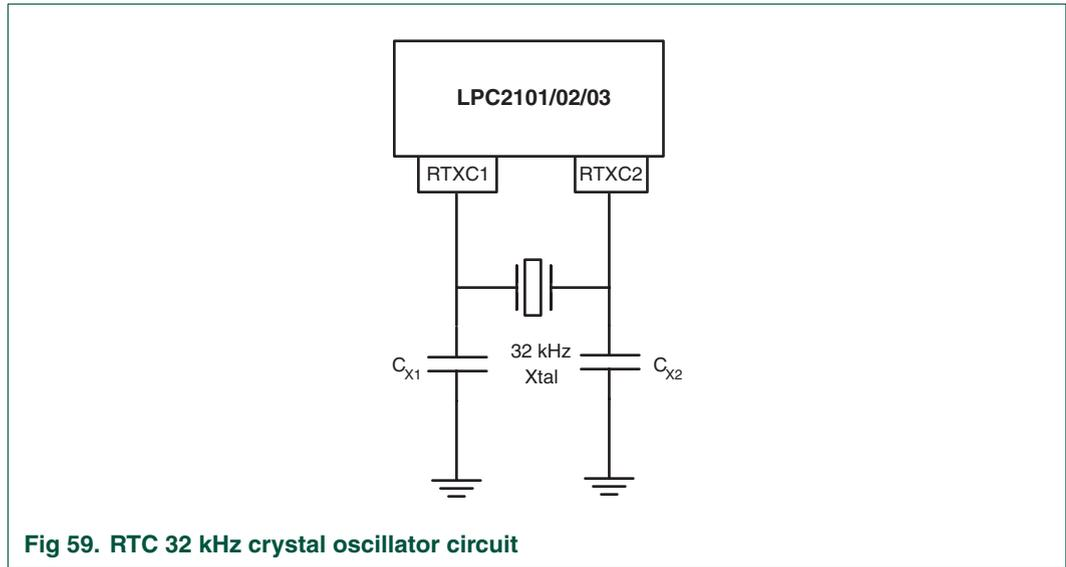
Fig 59. RTC 32 kHz crystal oscillator circuit
