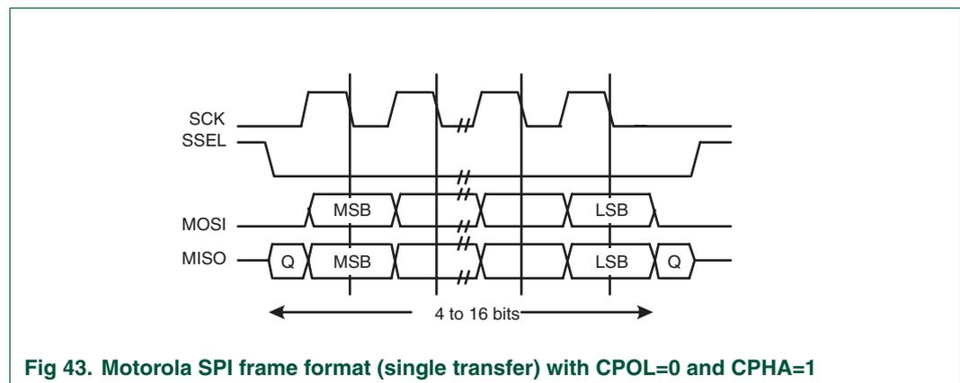
**Fig 43. Motorola SPI frame format (single transfer) with CPOL=0 and CPHA=1**
