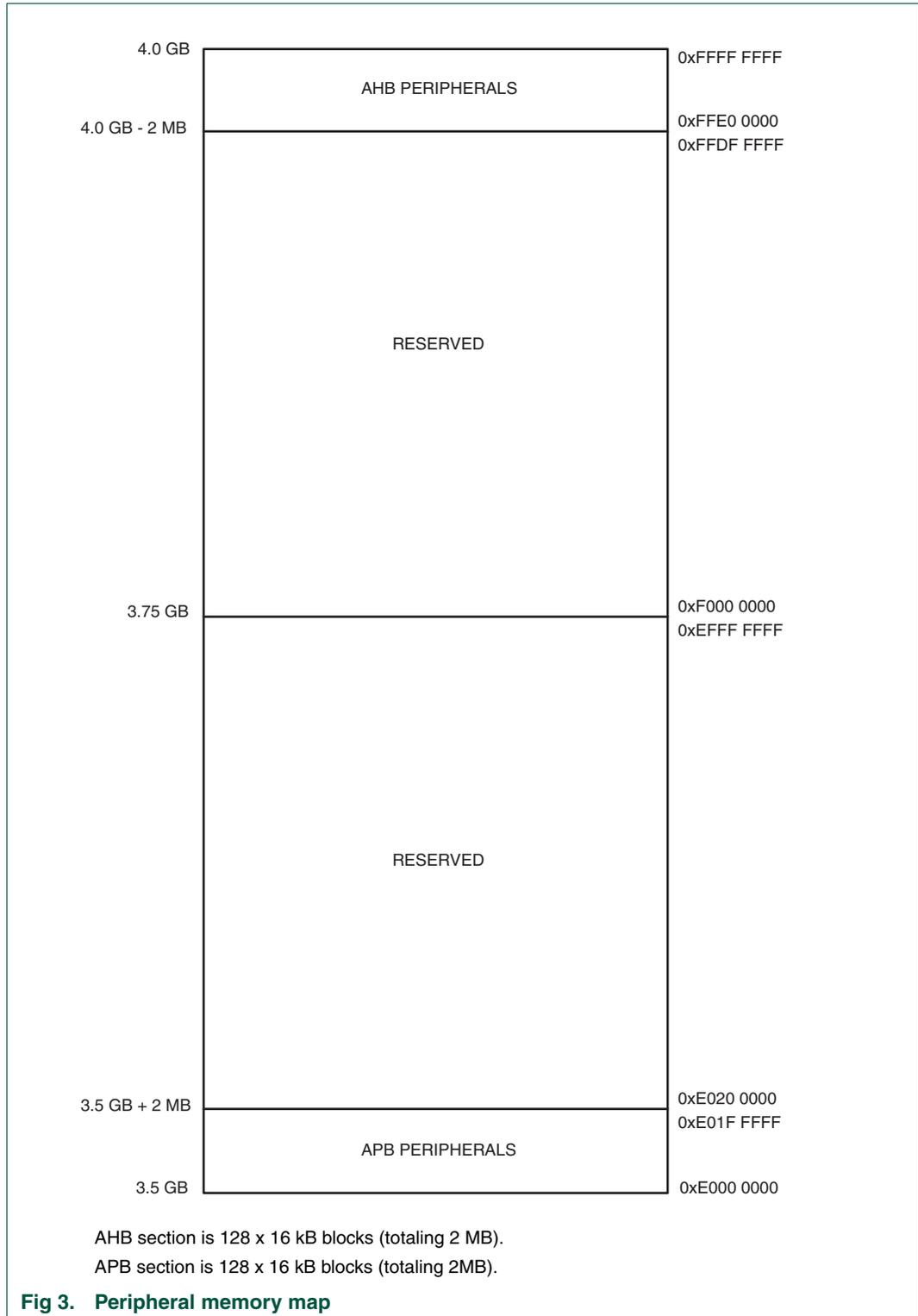
Figure 3, Figure 4, and Table 2 show different views of the peripheral address space. Both the AHB and APB peripheral areas are 2 megabyte spaces which are divided up into 128 peripherals. Each peripheral space is 16 kilobytes in size. This allows simplifying the address decoding for each peripheral. All peripheral register addresses are word aligned
