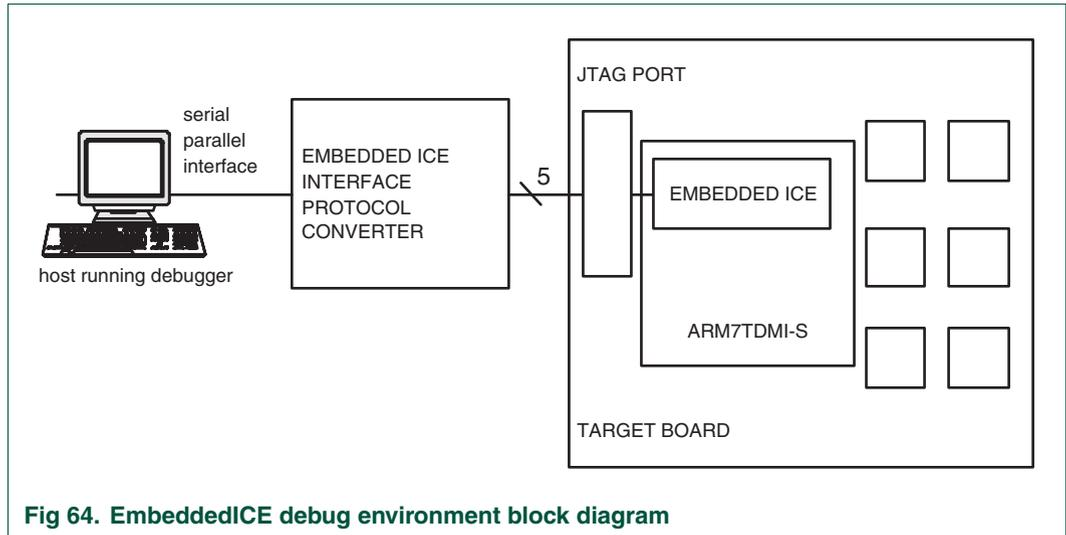
Fig 64. EmbeddedICE debug environment block diagram
