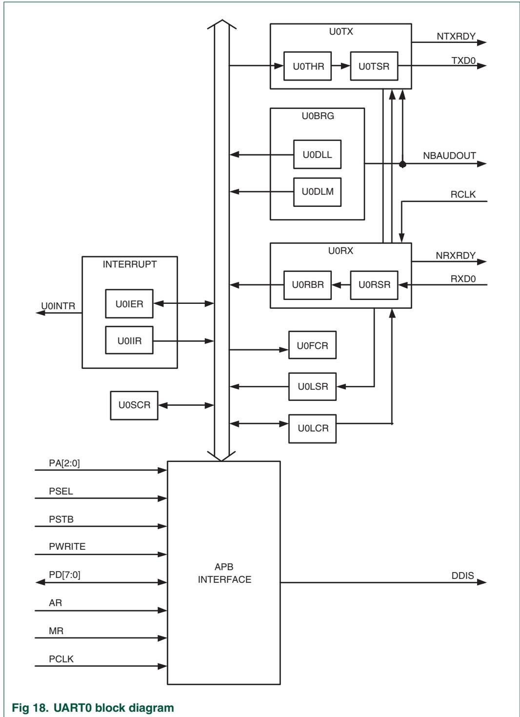
Fig 18. UART0 block diagram
