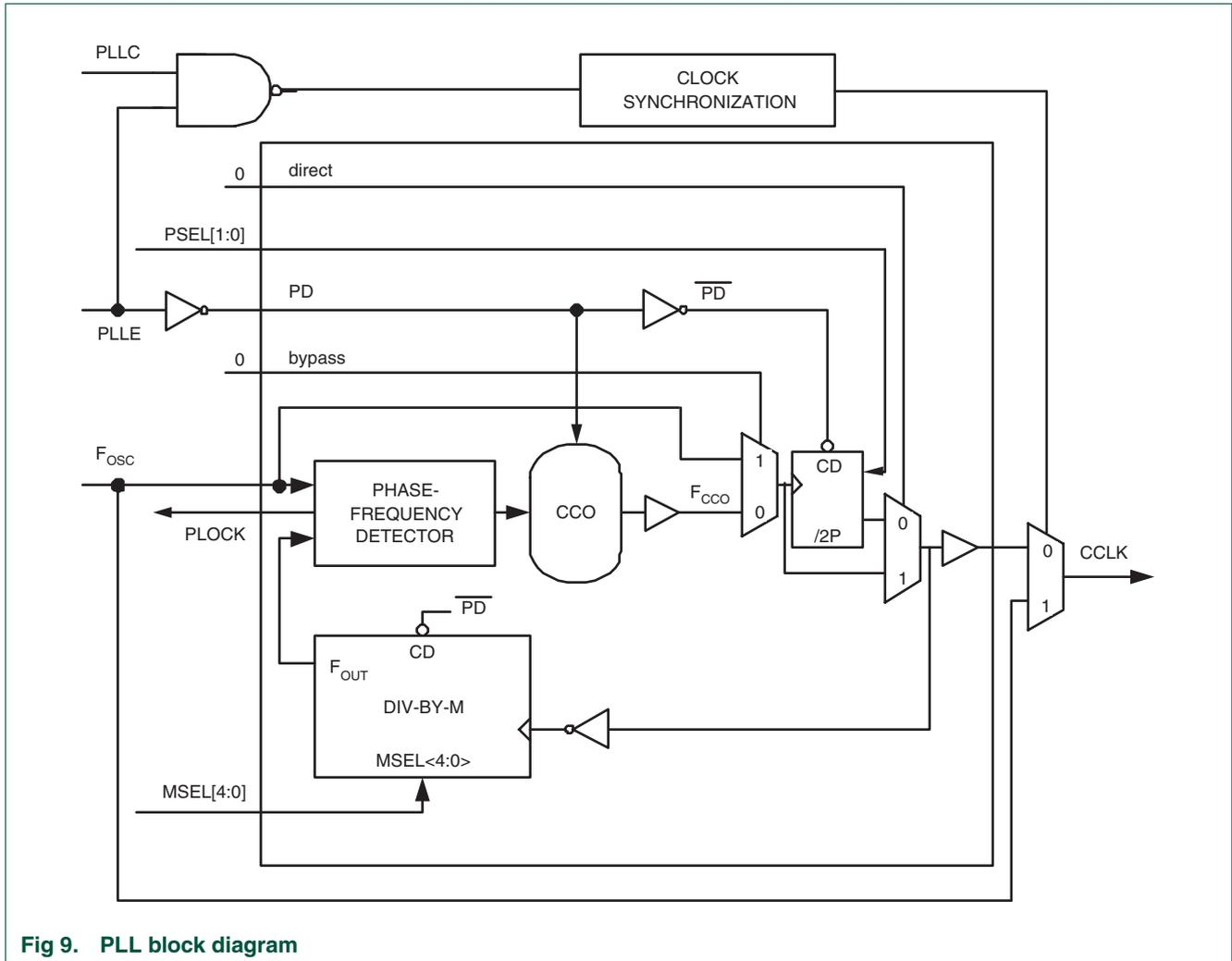
Fig 9. PLL block diagram
