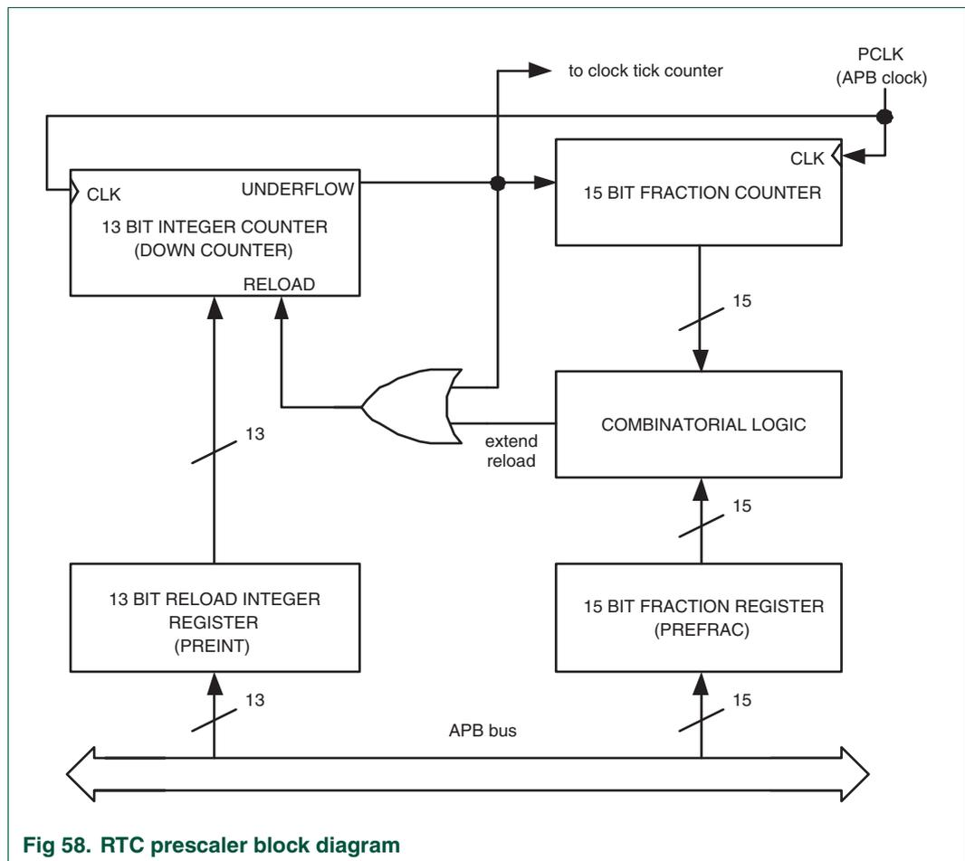
Fig 58. RTC prescaler block diagram
