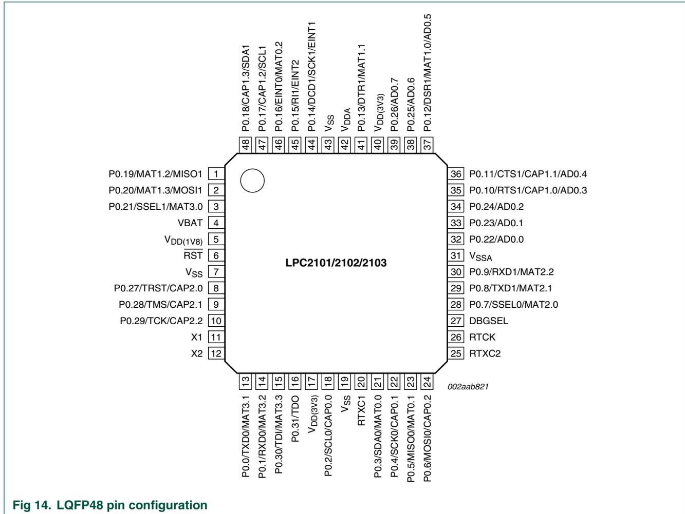
Fig 14. LQFP48 pin configuration
