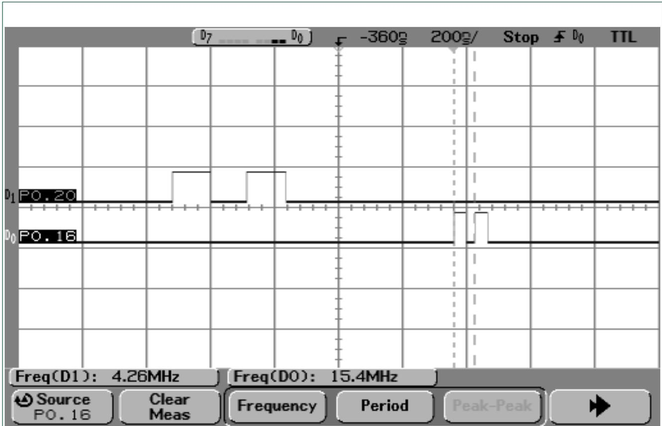
Fig 16. Illustration of the fast and slow GPIO access and output showing 3.5 x increase of the pin output frequency
