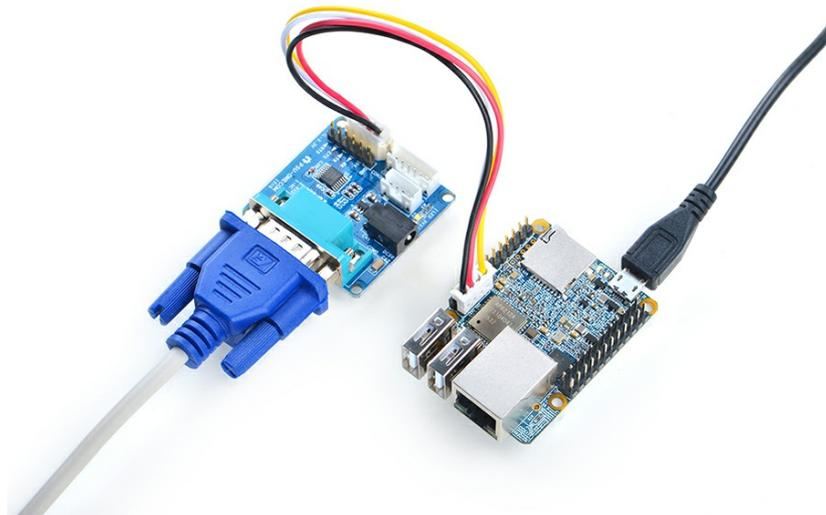
You can use a USB to Serial conversion board too. Make sure you use a 5V/2A power to power your NEO Plus2 from its MicroUSB port:
