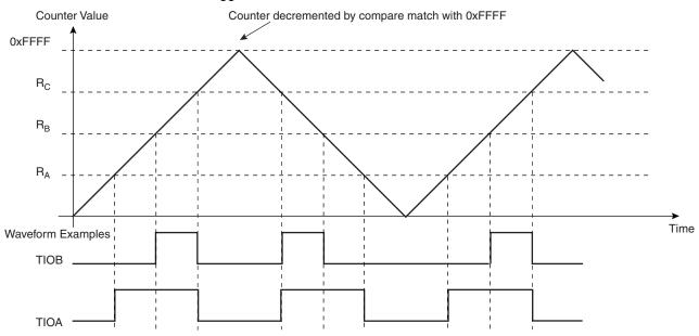
Figure 33-12. WAVSEL = 01 With Trigger
