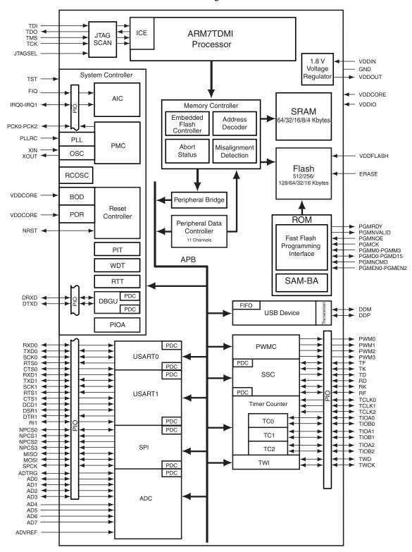
Figure 2-2. AT91SAM7S32/16 Block Diagram
