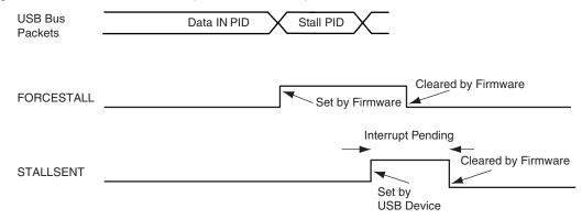
Figure 35-13. Stall Handshake (Data OUT Transfer)
