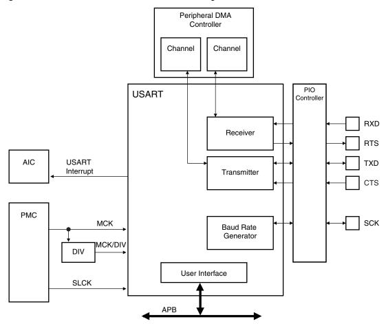
Figure 31-2. AT91SAM7S32/16 USART Block Diagram
