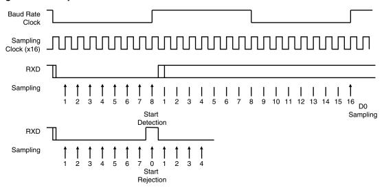
Figure 31-11. Asynchronous Character Reception
