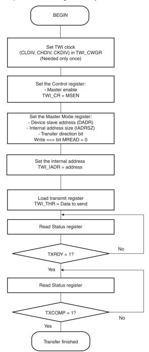
Figure 29-15. TWI Write Operation with Multiple Data Bytes with or without Internal Address
