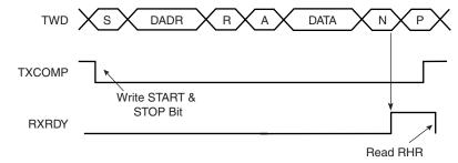
Figure 29-9. Master Read with Multiple Data Bytes
