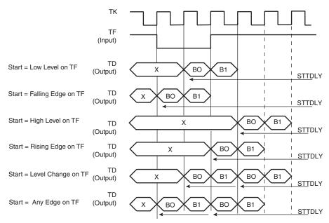
Figure 32-11. Receive Pulse/Edge Start Modes
