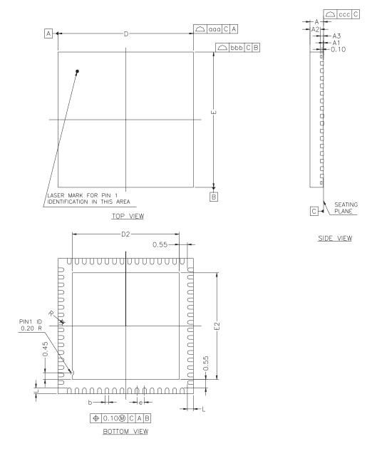
**Table 38-7.** 64-pad QFN Package Dimensions (in mm)
