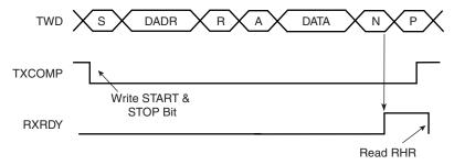
Figure 30-10. Master Read with Multiple Data Bytes
