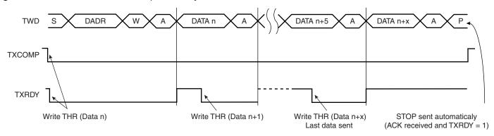
Figure 30-8. Master Write with One Byte Internal Address and Multiple Data Bytes
