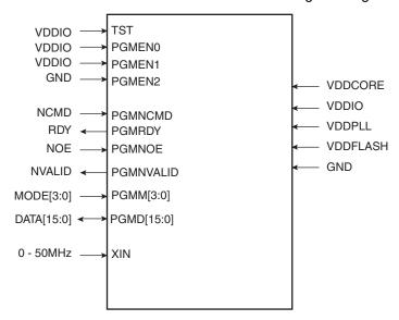
Figure 21-2. AT91SAM7S32/16 Parallel Programming Interface
