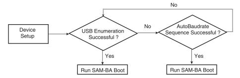
Figure 22-2. Boot Program Algorithm Flow Diagram without USB
