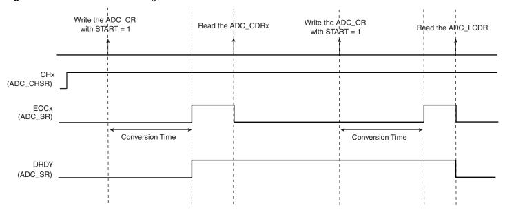
If the ADC\_CDR is not read before further incoming data is converted, the corresponding Overrun Error (OVRE) flag is set in the Status Register (ADC\_SR).
