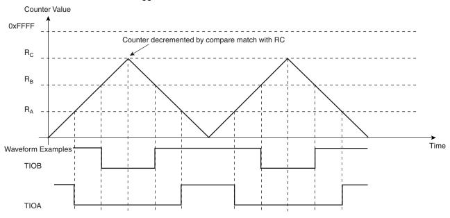
Figure 33-14. WAVSEL = 11 With Trigger
