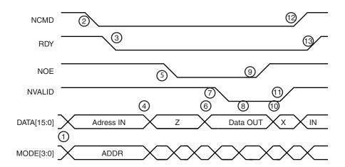
Figure 21-6. AT91SAM7S32/16 Parallel Programming Timing, Read Sequence
