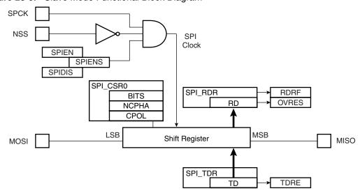
Figure 28-9. Slave Mode Functional Block Diagram
